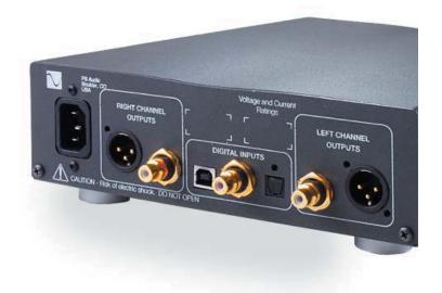
Plug either the RCA or the XLR outputs of the DLIII into a line level input on the preamp, integrated, Control Amplifier or Receiver. Do NOT plug the output of the DLIII into a phono or equalized input of any type.
