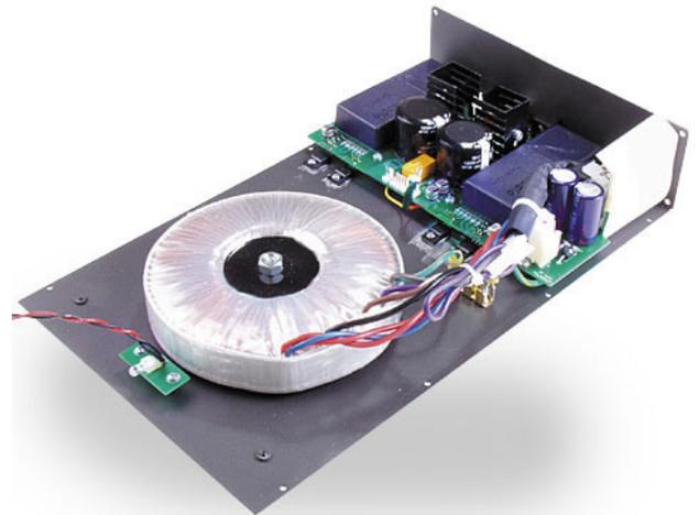
Hum may also be an issue with the GCHA if placed too close to a sensitive piece of equipment such as a phono preamplifier or turntable. The GCHA has an exceptionally large power transformer inside. This transformer can generate a fairly large magnetic field which can induce hum into sensitive equipment in close proximity.
