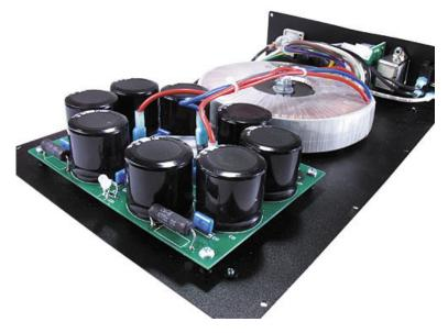
a fairly large magnetic field which can induce hum into equipment in close proximity. Be certain that the GCPS is placed as far away from other source and control equipment as possible.
