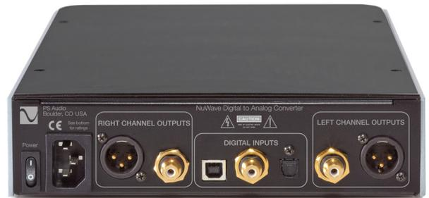
The preferred method of connection for a computer is USB. Connect the NWD to your computer using a well regarded high-end USB cable as short as possible. If you have a Mac the required driver is already installed. If you are using a Windows computer you will need to download and install the driver. See the Troubleshooting section for details.
